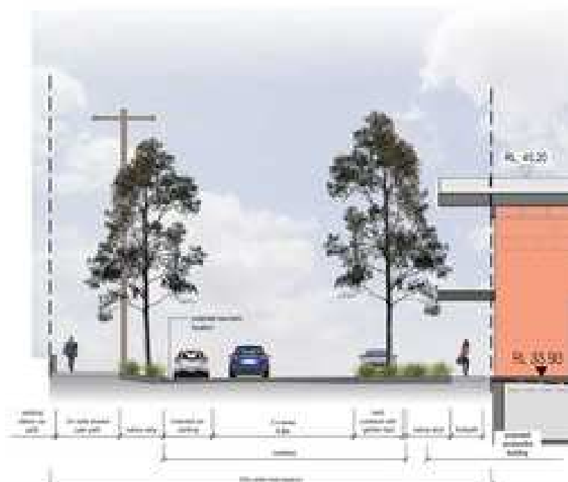
01 TYPICAL PROPOSED TURNHAM AVENUE SECTION 1:100 @ A1
